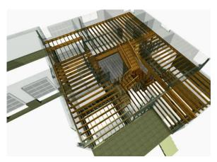
Figure 5: Detailed ArchiCAD model illustrating the framing sequence of the second floor. Student: Sara Jenson
